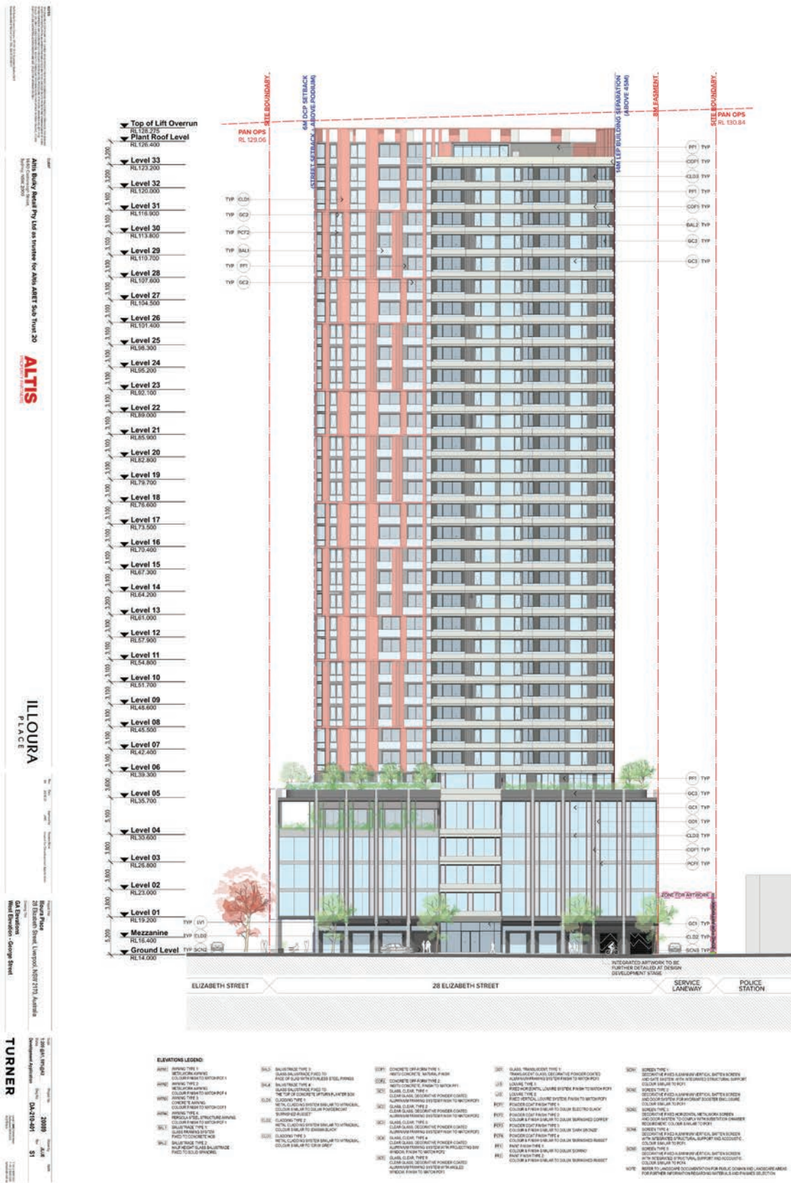
Figure 3: Elevation view of the proposed development (maximum height 128.275m AHD)
