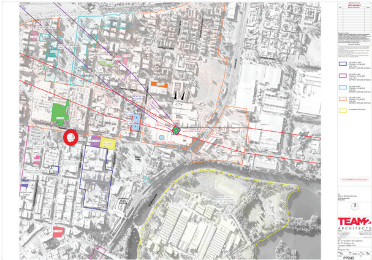
Figure 14: Old Western Flight Path (red) and updated Western Flight Path (purple) for Liverpool Hospital Helipad. The Altis site is indicated by the red marker.
